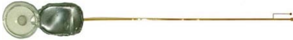
Fig. 14 A suprachoroidal (extraocular) implant for transretinal stimulation. The device consists of a receiver coil, hermetically sealed titanium package, and polyimide-based gold stimulation and reference electrodes (reproduced from Ref. [52])
