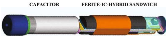
Fig. 4 Ceramic case microstimulator component arrangement. Reproduced from Ref. [4] with permission from IEEE
