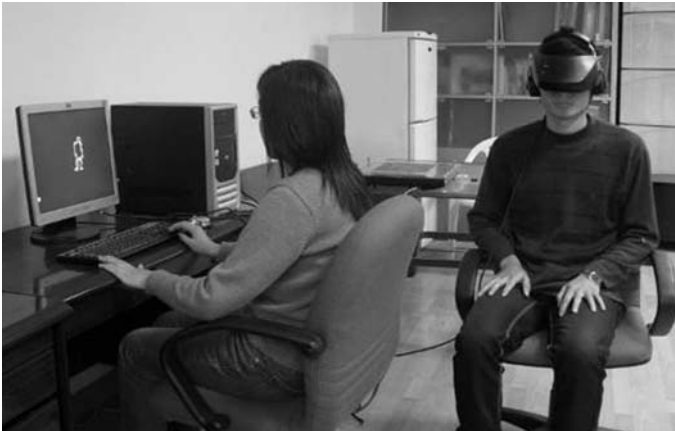
Fig. 22 The experimental scene of recognition of Chinese characters with a limited number of pixels: it was performed in a quiet and dark room to shield from ambient light. The pixelized images of Chinese characters with different resolutions ( 6 \times 6 , 8 \times 8 , 10 \times 10 , and 12 \times 12 ) were rendered on head-mounted display screen
