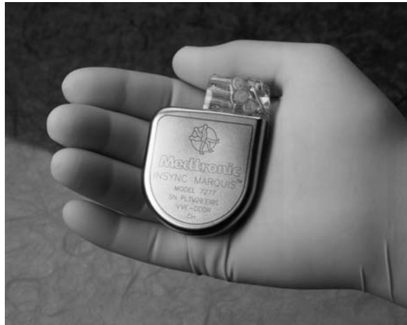
Fig. 13 A cardiac rhythm-timing (heart failure) pacemaker, InSync Model 7277, with a connector module accommodating 3 leads
