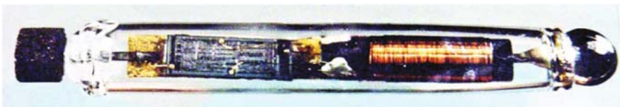
Fig. 1 Photo of the first version of the glass-encased RF-powered microstimulator Bion ® . From left to right : cylindrical shaped tantalum oxide coated open cell capacitor electrode attached via a tantalum stem which is hermetically sealed through a glass bead into the inside of the glass container. To the right of the stem is the 3 \mu\text{m} integrated circuit, followed by the coil-wrapped ferrite rod. On the right side is the iridium spherical-shaped electrode which is hermetically sealed to the glass case. (Reproduced from Ref. [4] with permission from IEEE)
