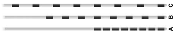
Fig. 8 Illustration of common contact spacings and spans observed in commercial products. As a dimensional reference, all contacts are 3 mm in length, and lead diameters are approximately 1.3 mm. Panels A, B, and C show 8-contact leads with center-to-center contact spacings of 4, 7, and 9 mm, respectively
