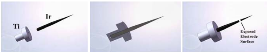
Fig. 11 This sequence shows an iridium pin welded to a titanium feed-through
