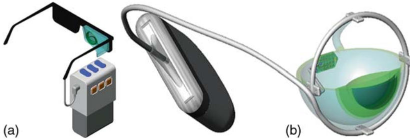
Fig. 9 The Second Sight Argus 16 electrode retinal stimulator implant. (a). The Argus 16 external system consisting of a pair of glasses housing a camera, a hip worn visual processing unit (VPU), and a primary coil that is magnetically attached to the scalp just behind the ear (where a secondary coil in a stimulator is implanted). (b) The electronic stimulator is implanted in the bone behind the ear. The cable connecting the electronics package to the array is tunneled up into the orbit where it encircles the eye and enters through a pars planar incision. The array is fixed on the epiretinal surface with a metal tack
