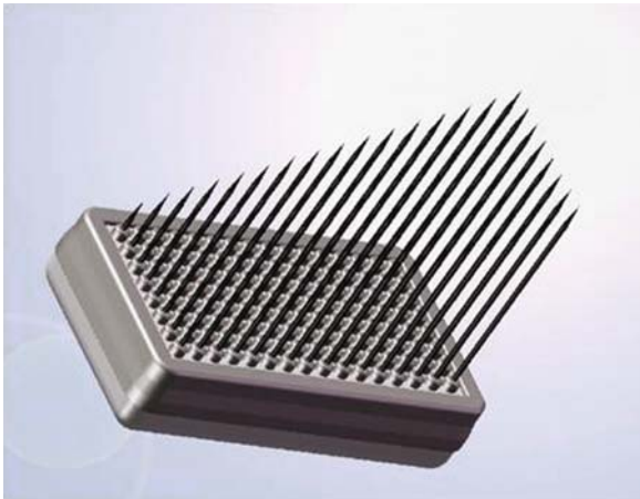
Fig. 12 Planned slanted bed of nails (SBON) showing a three millimeter thick electronics package in the form of the “bed”. The needles are brazed through a floor composed of a ceramic plate. The sides are titanium walls brazed to the side of the ceramic floor and ceramic ceiling. The titanium walls of the floor and ceiling are welded together
