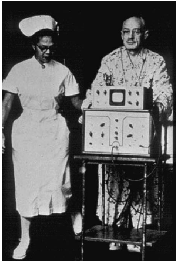
Fig. 2 Zoll AC powered pacemaker (PM-65) introduced in 1952. The distance the patient can travel is limited to the length of the power cord, which must be plugged into a wall outlet. Courtesy of The Heart Rhythm Foundation
